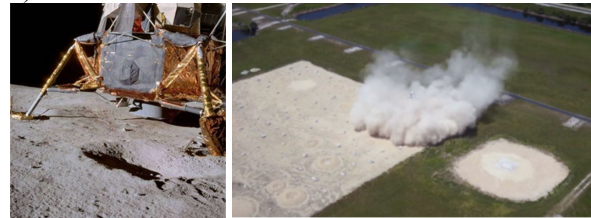
Fig 2. Apollo lander on Moon (left), and JSC Morpheus vehicle landing on lunar hazard field at KSC (right).
